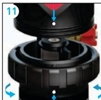
Replace the cartridge: the 3 cartridge splines align to the grooves in the bowl wall (10). Check that the 'O' ring is still seated correctly. Hold the bowl to the lid, line up the spigots on each then hand tighten the bowl locking collar (11). **Do not overtighten.**
