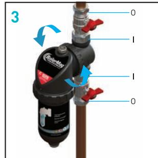
**UK INSTALLATION** Mark the pipe using the provided template as a guide (1). Cut out the marked section and remove burrs. Slide the isolation valve nuts and olives on to pipes (2). Loosely position isolation valves onto the outer nuts (O). Introduce the pre-assembled Boilermag unit ensuring the directional arrow follows the heating system flow. Ensure valve seals are fitted in place. Tighten the inner nuts (I) fully. Tighten
