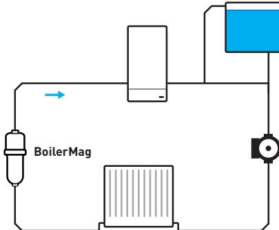
UK For best results install BoilerMag after the last radiator, prior to the boiler return. Ensure that there is adequate access to the BoilerMag for servicing and maintenance. To prevent frost damage do not install in locations where temperatures can fall below zero°C.
