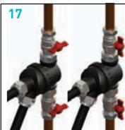
**SYSTEM FLUSHING** Flush adaptor is available separately from your BoilerMag supplier. (Product code: BMFA/1). Flush system. Unscrew port block collar to release BoilerMag (15). Fit flush adaptor to the port block, hand tightening port
